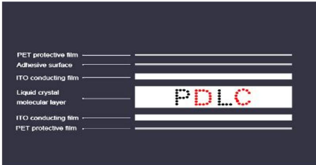
2,Smart PDLC film will become vaporous due to the disordered arrangement of liquid crystal molecules after turning off the power. On the contrary, when the power has opened,neatly organized molecules will make smart film present transparency.
