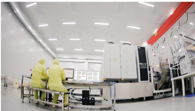
ITO Film Roll to Roll Coating Machinery from Germany
